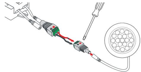
**3.** Insert Male Barrel Connector to Female Plug on Puck Light. Use Flat blade screwdriver to loosen screws on Male Barrel Connector. Insert wires, Red wire to (+), Black wire to (-), and tighten screws.
