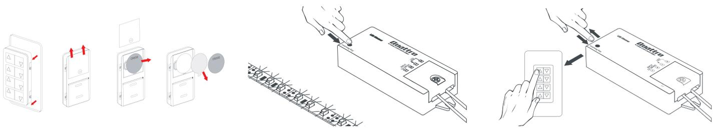
**1.** Remove Controller from back plate, slide battery compartment open, remove battery, and discard clear plastic tab. Reinsert battery, replace cover.
