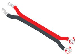
**1.** Cut a length of connection wire to run from Receiver to Tape Light location. Strip 1/4" insulation from both ends of wire, twist each wire, and fold stripped wires in half on both ends.
