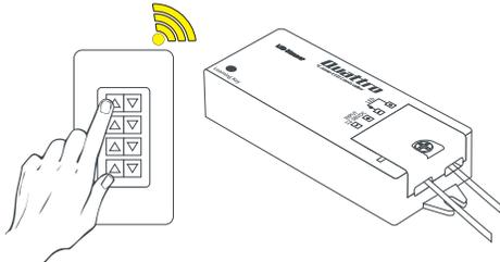
**4.** Turn on 120V AC to Power Supply and pair Receiver to Controller.
