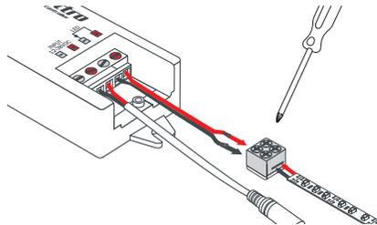
**5.** Use #1 Phillips to loosen the 4 terminal screws on 8MM-EZ Connector. Peel 1/2" of the adhesive protector from back of LED tape light, insert into connector, evenly tighten screws. Insert wires from Receiver into terminals, Red wire to (+) side of tape, Black wire to (-) side of tape; tighten screws.
