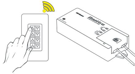
**2.** Turn on 120V AC to Power Supply and pair Receiver to Controller.
