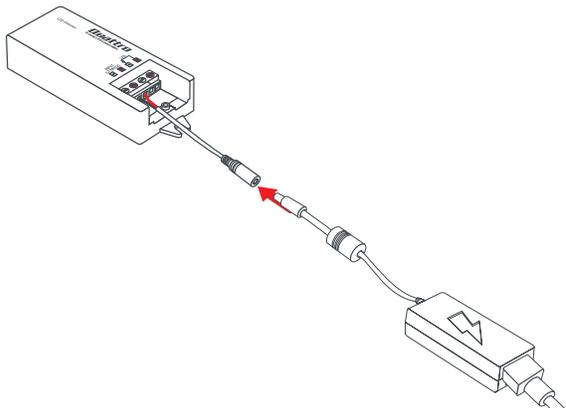
Insert the Male Barrel Connector on the Power Supply into the Female Plug Cable on the Receiver.
