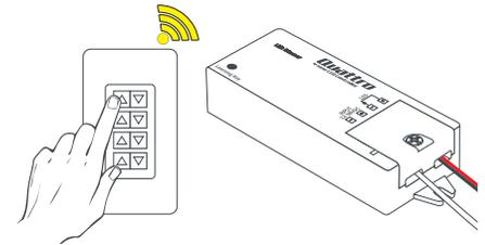
**6.** Turn on 120V AC to Power Supply and pair Receiver to Controller.
