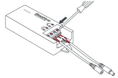
**3.** Use a flat blade screwdriver to loosen terminals for the Male Plug and remove.
