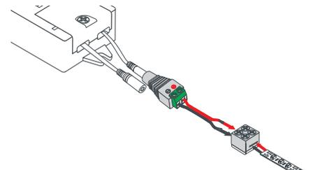
**3.** Use #1 Phillips to loosen the 4 terminal screws on 8MM-EZ Connector. Peel 1/2" of the adhesive protector from back of LED tape light, insert into connector, evenly tighten screws. Insert wires from Receiver into terminals, Red wire to (+) side of tape, Black wire to (-) side of tape; tighten screws.
