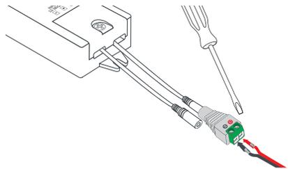
**2.** Insert Male Plug on Receiver into Female Barrel Connector. Use Flat blade screwdriver to loosen screws on Female Barrel Connector. Insert wires, Red wire to (+), Black wire to (-), and tighten screws.
