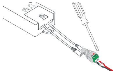
**2.** Insert Male Plug on Receiver into Female Barrel Connector. Use Flat blade screwdriver to loosen screws on Female Barrel Connector. Insert wires, Red wire to (+), Black wire to (-), and tighten screws.
