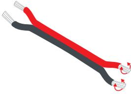
**1.** Cut a length of connection wire to run from Receiver to Tape Light location. Strip 1/4" insulation from both ends of wire, twist each wire, and fold stripped wires in half.
