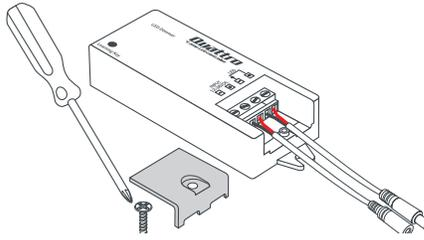
**2.** Use #2 Phillips to loosen screw and remove cover from Receiver.
