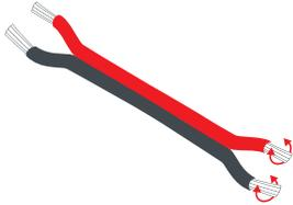
**1.** Cut a length of connection wire to run from Receiver to Puck Light location. Strip 1/4" insulation from both ends of wire, twist each wire, and fold stripped wires in half.
