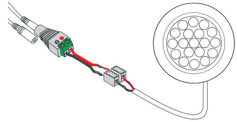
**3.** Cut Female Plug on Puck Light and insert wires, matching Red wire to Red, Black wire to Black into EZ-WSC Connector.
