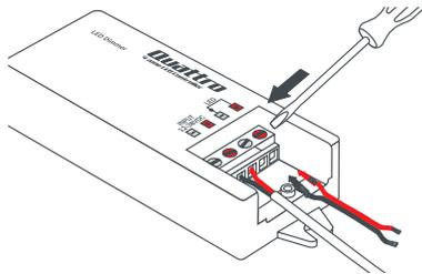
**4.** Insert one end of stripped wires into Receiver LED terminals, Red wire to (+) and Black wire to (-) terminals. Tighten screws.
