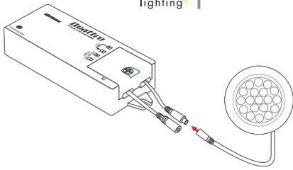
**1.** Insert Male Plug on Receiver into Female Plug on Puck Light.
